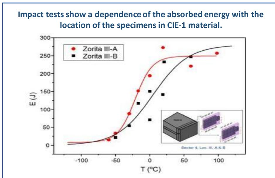
Figure 1 – Charpy V-notch transition curves of material CIE-1 (Zorita, MnMoNi) for same location
