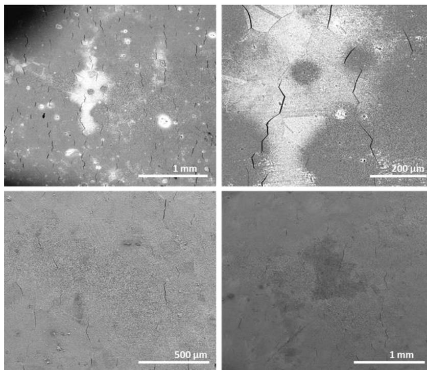
Figure 2 – SEM images showing IASCC on the proton irradiated 316L SS specimen surface post-4-point-bend SCC testing.
