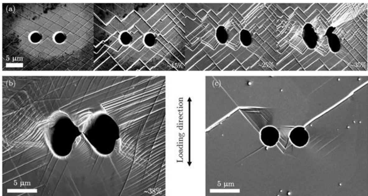
*Figure 3 – Typical observations of voids coalescence in the material exhibiting dislocation channeling deformation mode.*
