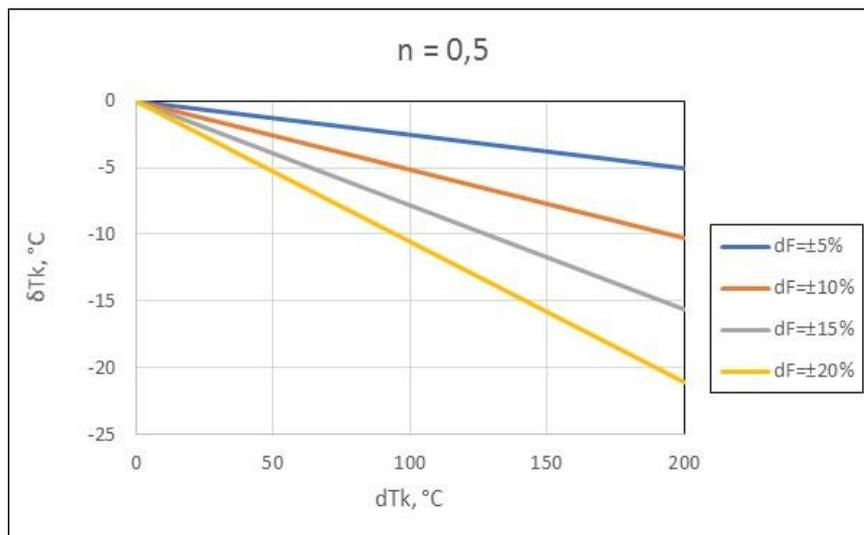
*Figure 1 – Effect of the different maximum scatter of neutron fluence in individual specimens in a surveillance set on the difference in transition temperature for different level of embrittlement ( $dT_k$ ) and constant slope of Embrittlement Trend Curve ( $n=0.5$ )*
