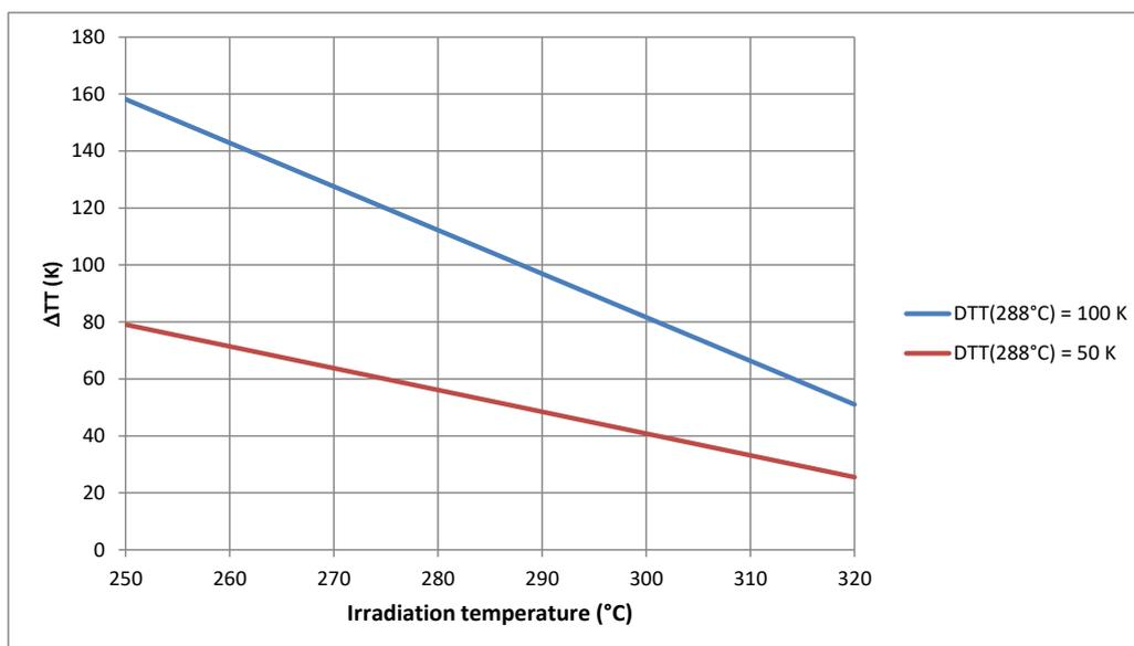
Figure 3 – Effect of irradiation temperature on transition temperature shift  $\Delta TT$
