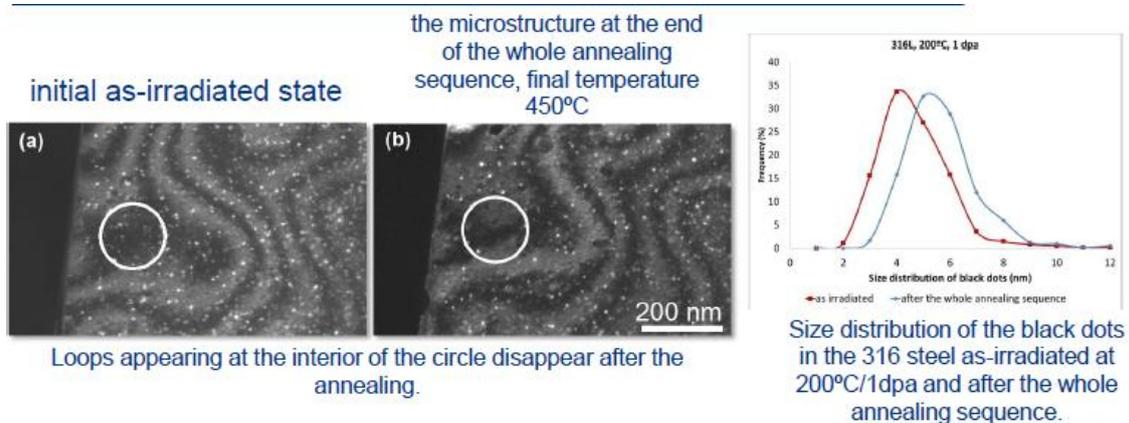
Figure 2 – In situ TEM post irradiation annealing of ion irradiated stainless steel (CIEMAT, CVR)
