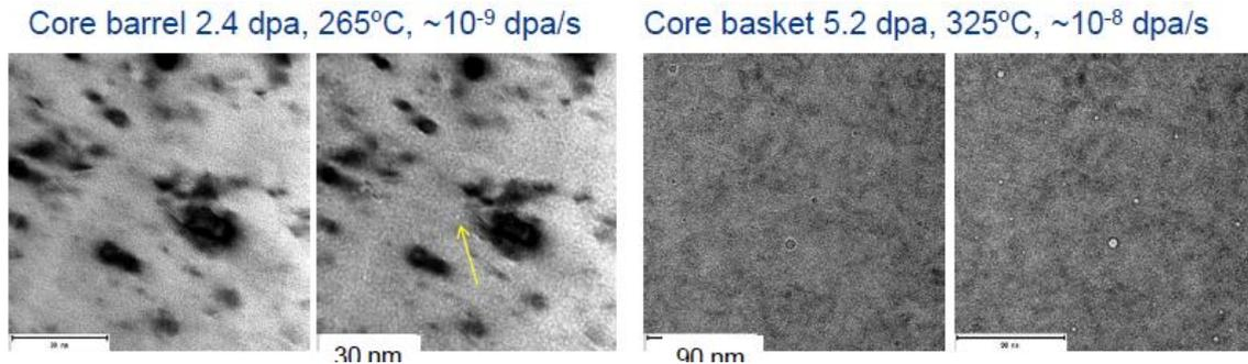
Figure 1 – TEM examination of neutron irradiated stainless steel (CIEMAT, CVR)
